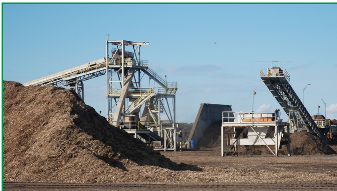
Figure 2. Conveyors processing woodchips for renewable energy at IVRR's facility in Imperial, CA.
